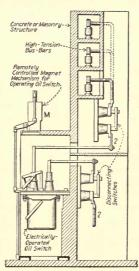
Fig. 236.—Remote-control oil switch in masonry-cell mounting.
